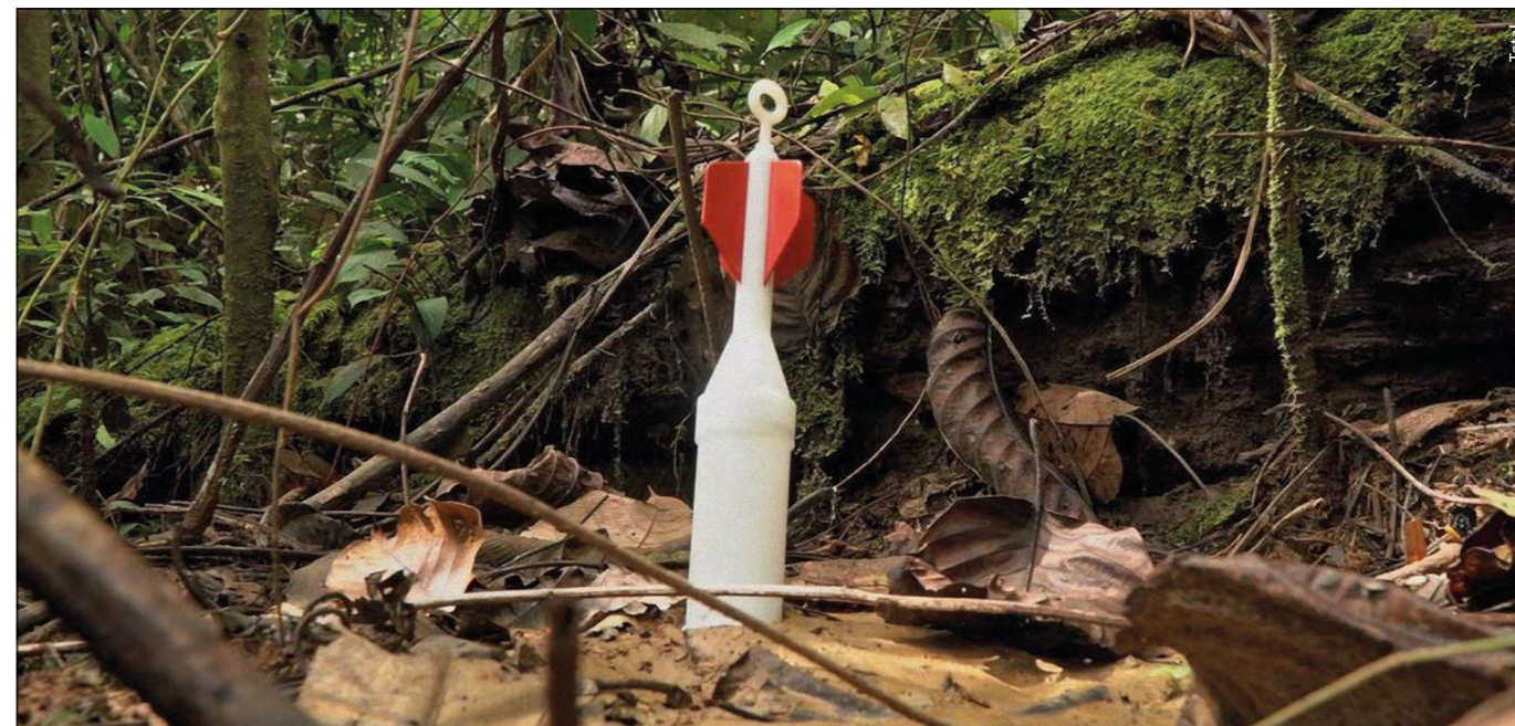
In the pilot project the DARTs successfully embedded themselves in the ground and transmitted data. They are designed to be biodegradable, leaving no trace after the survey is completed.
