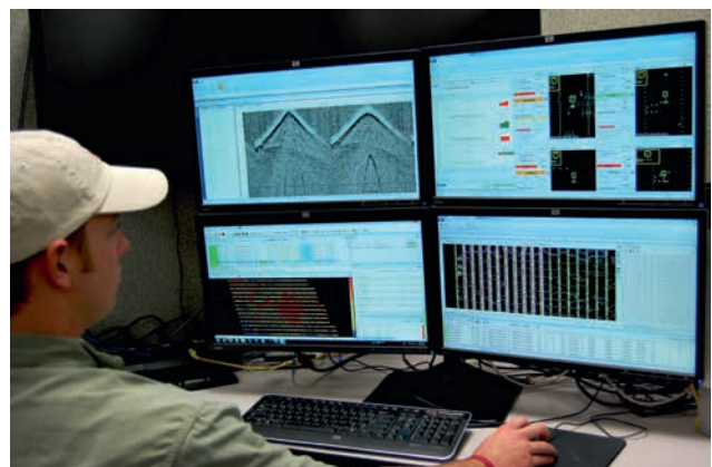
Figure 3 Wireless Seismic real-time multi-screen display of the seismic record, survey map, noise levels, status of the individual modules and other parameters.
