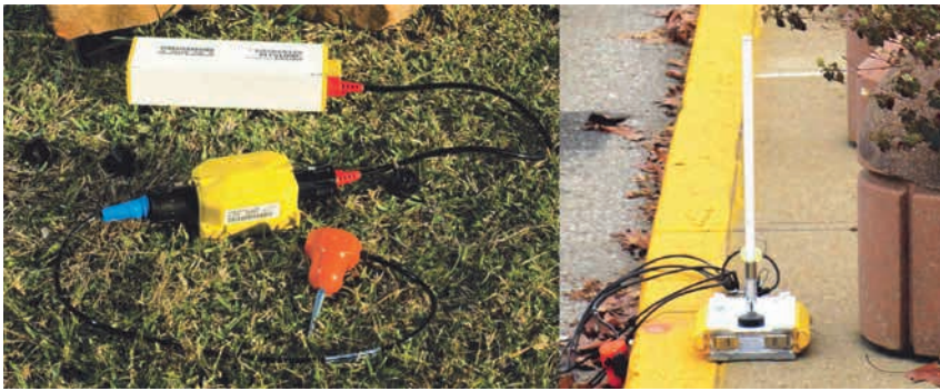
Figure 1 Left: Geospace GSR, an early market leader in the autonomous node market segment. Right: Wireless Seismic RT2 delivers seismic data to the dog house in real time over a radio link.
