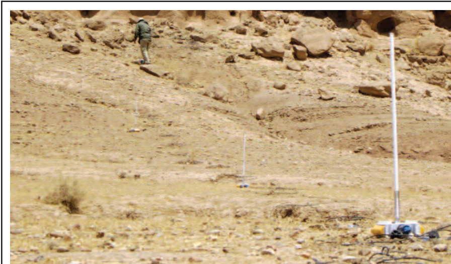
The first widely accepted cable-free seismic systems were introduced a decade ago, and since have grown to more than 25 percent of the world seismic acquisition market. The early units were self-contained systems that digitized data from a sensor and saved them in memory. The next generation of data acquisition systems should be able to leverage numerous advances in wireless transmission, and power and data storage, to further improve efficiency, reliability and overall recording capabilities.
