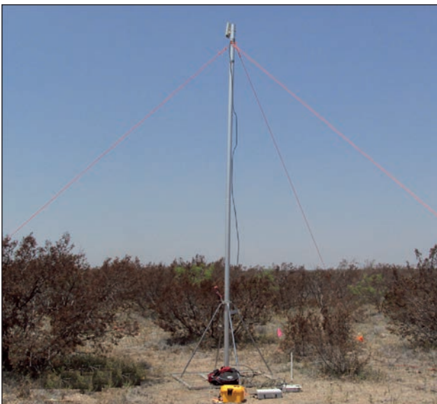
Figure 4 Line Interface Unit with transportable antenna.
