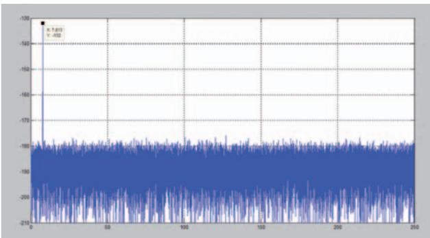
Figure 5 Single sine, gain 64, 250 Hz bandwidth, 32 bit output.
